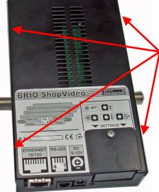
Close base unit and fix it with four screws on the edges of the case.
