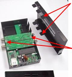
On the base unit top cover break down the protective caps in connector's place of installed video channel module.
